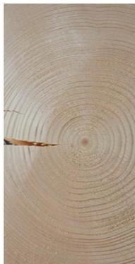
**Bild 7:** Schwindriss
